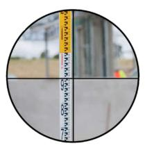
Horizontal and vertical cross-hairs allow for vertical and horizontal alignment.
