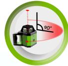
Vertical Plumb Spot Self Levelling (90° to horizontal plane)
